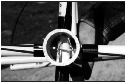
Fig 58 — An end-on view of the top of the QHA prior to soldering the loops and installing the PVC cap.
